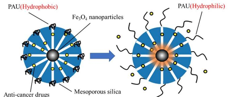
Figure 1. Schematic of MMS-PAU and drug release
